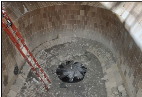
Top view of re-pulper "pit" where defective paper is ground by the blades.
